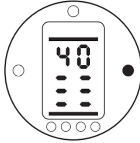
Fig. 3.5. 40% of maximum rated pressure, Fully Open.
