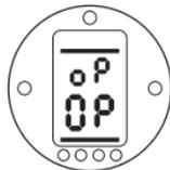
Press the + or – keys until the required output is shown on the measuring device for the Open limit position.
