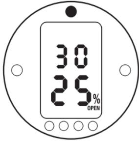
Fig. 3.4. 30% of maximum rated pressure, 25% Open.
